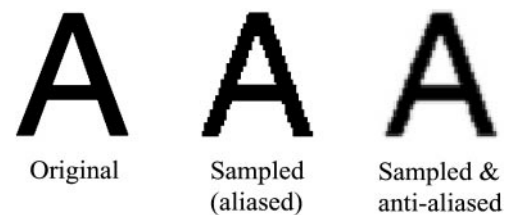
Figure 1. Aliases and antialiasing. Left , A high-resolution image with smooth edges is shown. Middle , The same image sampled with relatively low-resolution interpixel distance appears to have new features with high spatial frequency (the jagged stair steps). These “aliases” are introduced when the distance between adjacent sensors (pixels in this case) is insufficient to render the high-resolution image. Right , The same image sensed with the low-resolution pixels of the middle panel and antialiased is shown. Antialiasing includes a low-pass filter that removes the spurious alias features from the image and therefore may also (as in the present instance) eliminate some high-spatial frequency detail from the original image. The corresponding potential introduction of artifacts into array-sampled physiological data can be removed by the same antialiasing method (see Fig. 2 legend below) and will correspondingly eliminate some fine (high-spatial frequency) detail from the data.
