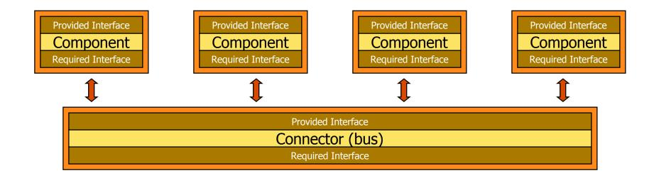
Connections are provided by connectors, with communication via events on the software bus
