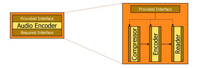
Compressor IS-COMPONENT-OF Audio Encoder
