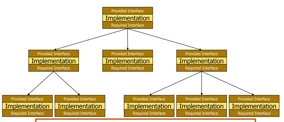
Abstraction through the use of provided/required interfaces Modularity through the use of components Low coupling through the use of hierarchies High cohesion through the use of coherent implementations
