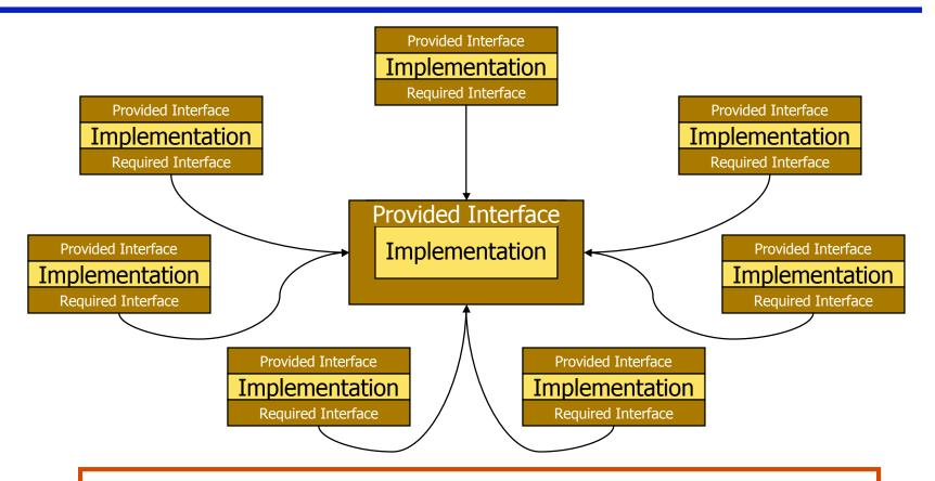
Abstraction through the use of provided/required interfaces Modularity through the use of components Low coupling through the use of a central "blackboard" High cohesion through the use of coherent implementations
