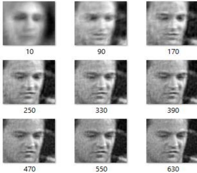
Figure 5: Faces reconstructed with different numbers of Eigenvectors
