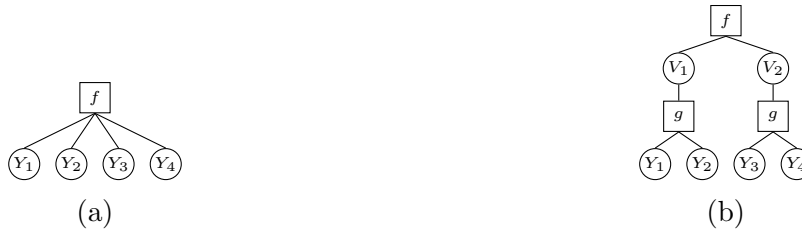
Figure 2.4: Decomposition of large constraint factors. (a) A global constraint factor f , defined over four variables for the sake of illustration. (b) By introducing two auxiliary variables, V_1 and V_2 , we can decompose the constraint into three factors defined over two or three variables each.
