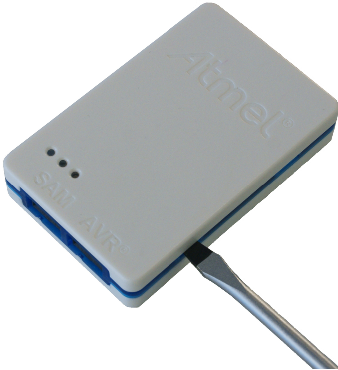
Figure 2-13. Opening the Atmel-ICE (2)
