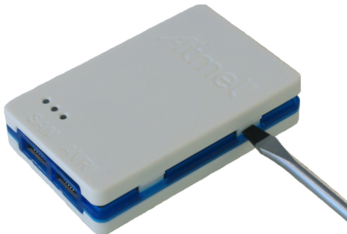
Figure 2-13. Opening the Atmel-ICE (2)
