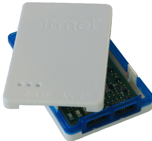
Figure 2-14. Opening the Atmel-ICE(3)
