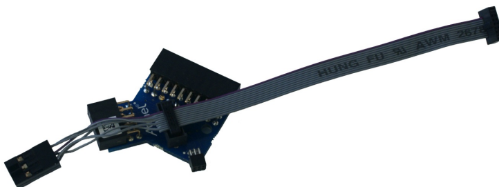
Figure 2-9. Atmel-ICE Cable Connection
