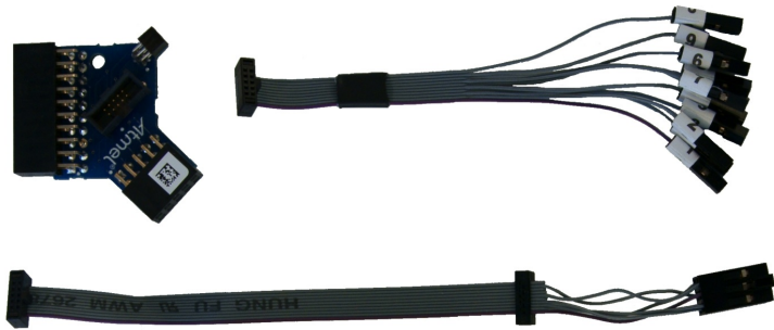
Figure 2-4. Atmel-ICE Adapter Kit Contents
