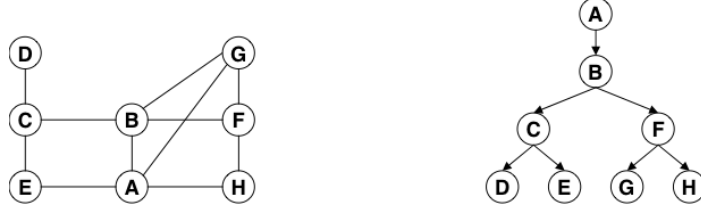
Figure 1: Example constraint network and pseudo tree. The constraints are C_1 = F \vee H, C_2 = A \vee \neg H, C_3 = A \otimes B \otimes C, C_4 = F \vee G, C_5 = B \vee F, C_6 = A \vee E, C_7 = C \vee E, C_8 = C \otimes D, C_9 = B \vee C . The ordering for the pseudo tree is d = (A, B, C, D, E, F, G, H) . (Taken from [4].)
