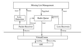
Figure 1: Block Diagram of Reliability Implementation
