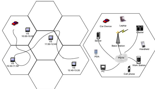
**Fig. 1.** System environment: (a) An example of providing service for a mobile client by Volunteer Servers available in grid system, (b) Possible components within a cell
