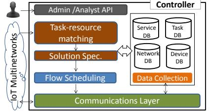
Fig. 1. IoT controller Architecture
