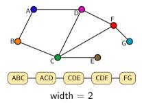
Pathwidth of a graph is smallest width of any path decomposition
