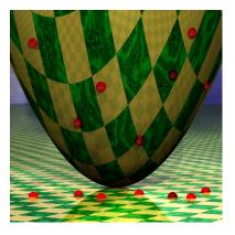
Therefore, lower hull faces (sets of points touched by boundaries of empty lower halfspaces  $\iff$  Delaunay edges and triangles (sets of points touched by empty circles
