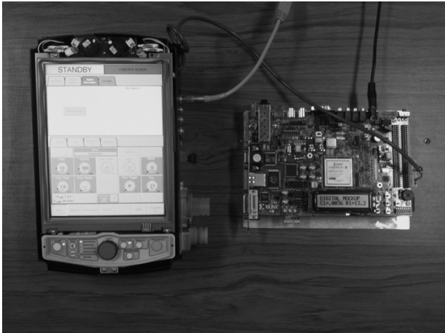
Figure 5: Ventilator device connected to digital mockup implemented on a Xilinx Virtex5 FPGA.
