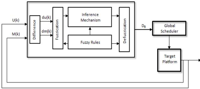
Figure 4: Internal structure of the feedback controller
