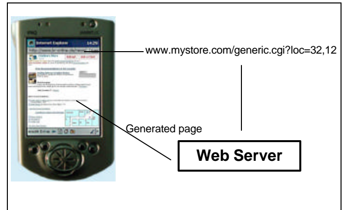
Figure 3: Snapshot of the LAWS Browser after the user attempts to be located
