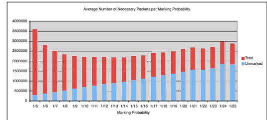
Fig. 10. Average packet frequencies needed to identify 1000 leaves in a binary attack tree  $T$  with depth 10, for various marking probabilities. Each frequency is averaged over 100 runs of the experiment.
