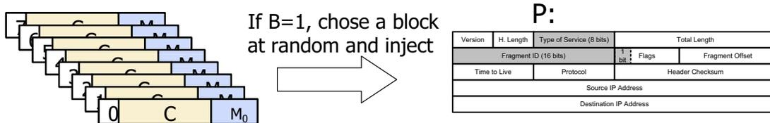
Fig. 3. The block injection process. Potentially-reusable bits are shown shaded.
