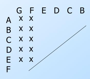
Start with marks for the pairs with one of the final states F or G.
