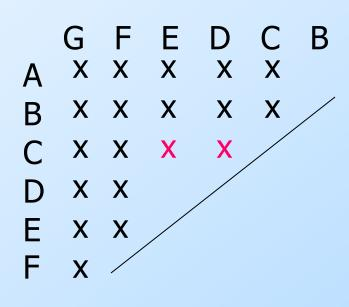
[C, D] and [C, E] are marked because of transitions on b to marked pair [F, G].
