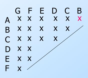
[A, B] is marked because of transitions on r to marked pair [B, D].
