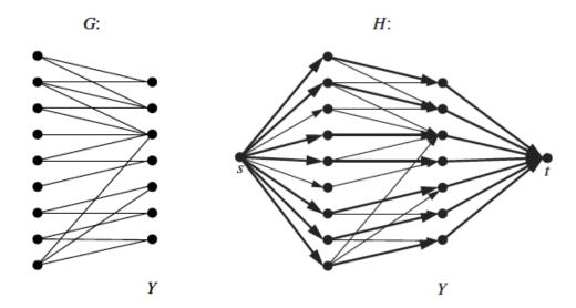
Figure 16.11: (a) A bipartite graph G. (b) Flow network H derived from G and a maximum flow in H; thick edges have unit flow and other edges have zero flow.
