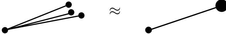
Figure 1: The far-field effect from several point charges can be approximated as a single function capturing their net effect, rather than requiring that each contribution be calculated individually.
