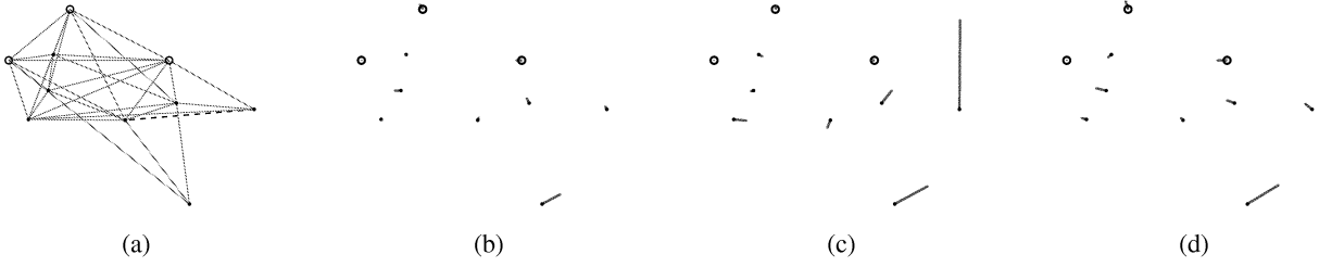
Fig. 5. (a) A small (10-sensor) graph and the observable pairwise distances; calibration is performed relative to the location of the sensors shown in green. One distance (shown as dashed) is highly erroneous, due to a measurement outlier. (b) The MAP estimate of location, discarding the erroneous measurement. (c) A nonlinear least-squares estimate of location is highly distorted by the outlier; (d) NBP is robust to the error by inclusion of a measurement outlier process in the model.
