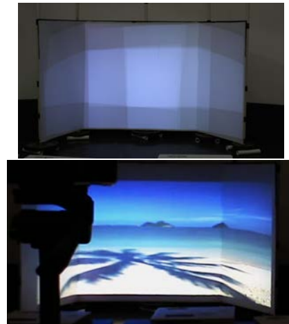
Figure 10: Top: A picture of our CAVE setup with the projectors overlapping on the edges. Bottom: Geometric registration on our CAVE setup. The calibrating camera is visible in the top-left corner of the picture.
