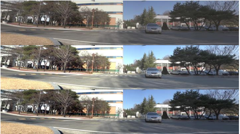
Fig. 4. Panorama stitched using five camera views with automatic color reference selection. ( Top ): Default reference I_1 , ( Middle ): Setting I_5 as reference, ( Bottom ): Setting I_4 as reference.
