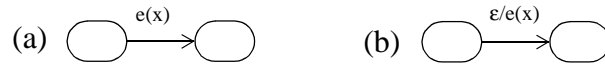
FIGURE 14. (a) A CSP event with input data, e?x , is modeled in UML state machines as a state transition event with no action. (b) A CSP event, e , with output data, e!x , is modeled as a null state transition event that results in action e .
