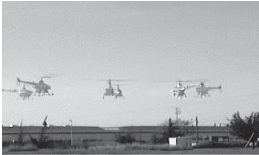
Figure 21.10 FILES: figures/heliComposite.eps (Tue Nov 3 16:23:02 2009). Superimposed time-lapse images of an autonomous helicopter performing a very difficult “nose-in circle” maneuver. The helicopter is under the control of a policy developed by the PEGASUS policy-search algorithm. A simulator model was developed by observing the effects of various control manipulations on the real helicopter; then the algorithm was run on the simulator model overnight. A variety of controllers were developed for different maneuvers. In all cases, performance far exceeded that of an expert human pilot using remote control. (Image courtesy of Andrew Ng.)
