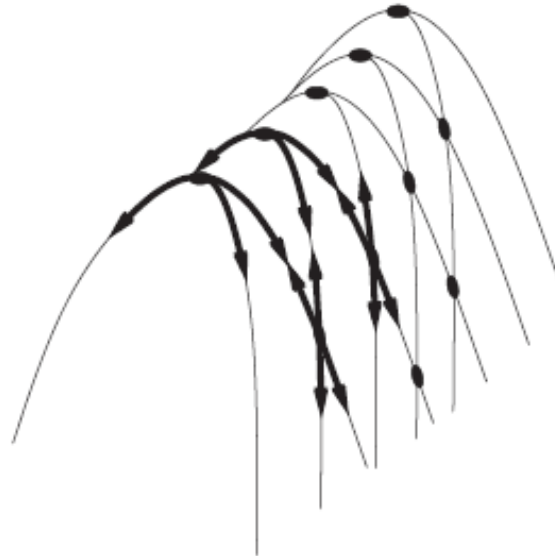
Figure 4.4 FILES: figures/ridge.eps (Tue Nov 3 16:23:29 2009). Illustration of why ridges cause difficulties for hill climbing. The grid of states (dark circles) is superimposed on a ridge rising from left to right, creating a sequence of local maxima that are not directly connected to each other. From each local maximum, all the available actions point downhill.
