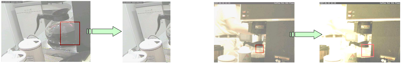
Figure 6. The initial and the resulting bounding rectangle for the two cameras.
