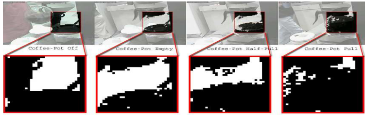
Figure 1. The 4 different states in our example. The black/white cells represent dark/bright average pixel color.
