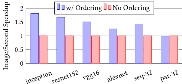
Figure 3: Throughput speedup of ordering algorithms for different models. Higher the better. Seq-32 is a 32-layer sequential model (similar to Recurrent models.) Par-32 is a 32-layer parallel model.
