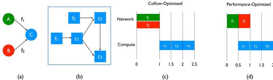
Figure 1: Importance of understanding application objective: (a) Coflow with two component flows.  $f_1$  and  $f_2$  (size 500Mb each) share a 1Gbps bottleneck link. (b) Computation model at  $C$  has 3 operations,  $c_1$ ,  $c_2$ , and  $c_3$  with dependencies between flows and computations as shown. Each computation operation takes 0.5s to execute. Completion times with (c) coflow completion time-optimized transfers and (d) application objective-based optimization for transfers.
